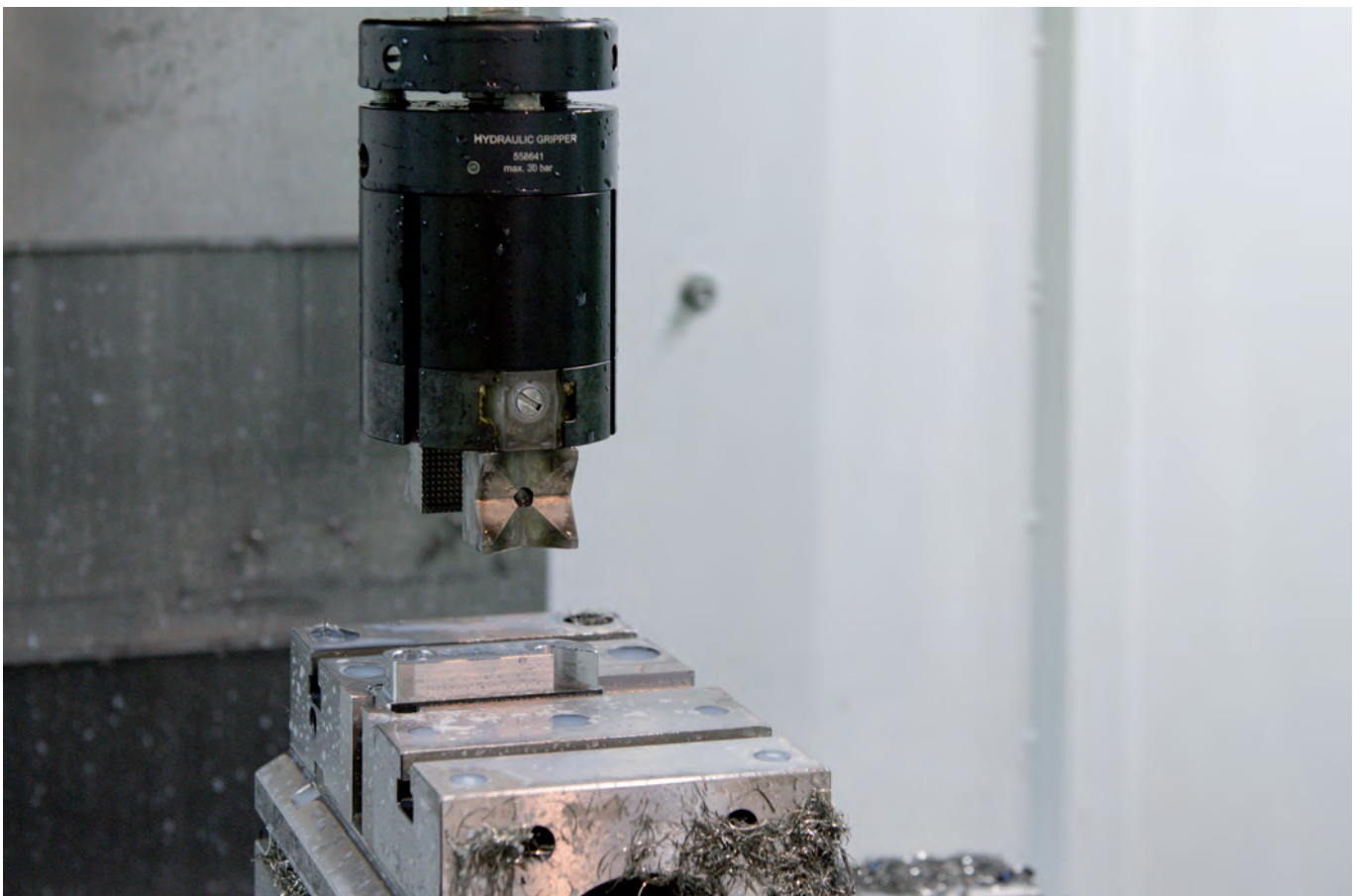
Low-cost automation, easy to implement. The AMF gripper is unloaded from the tool storage of the milling machine and transports the workpieces between the clamping system and workpiece storage before and after processing.
