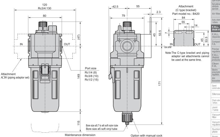
Note: The C-type bracket and piping adaptor set attachments cannot be used at the same time.
