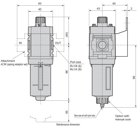
Attachment (C type bracket) Part model no.: B120
