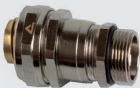
ISO cable-hose fitting, compact, male, double seal acc. EN 45545-2, HL1 / HL2 / HL 3, table R22 and R23 (incl. brass connection set)
