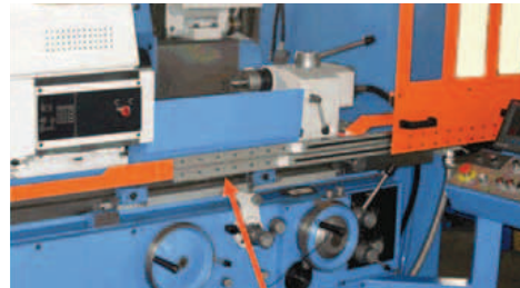
drylin® NT LM in guard door adjustment in machine tool
