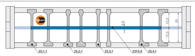
By standard vertical separators are assembled every 2<sup>nd</sup> E-Chain® link
