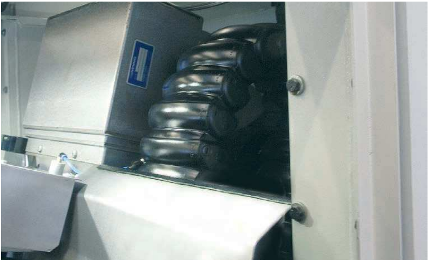
Despite the restricted installation space, the RX e-tube is used in this compact turning machine with Reverse Bend Radius (RBR)
