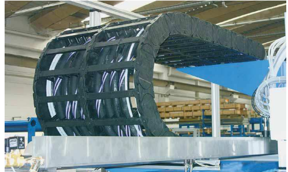
E4.1 as a noise-optimised version with extension links. Unsupported application with high fill weight. Harnessed with rigid hydraulic hoses. The max. noise level can be reduced up to 9dB(A) using the optional rubber dampers
