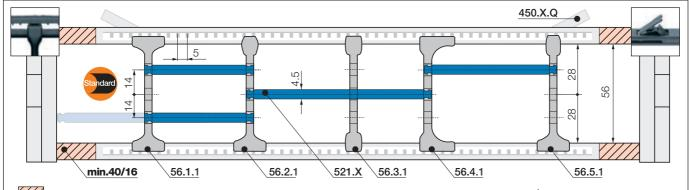
Note: please be aware of the minimum lateral gap to the side links! e-tube: 40 mm | e-chain®: 16 mm As standard igus® separators should be fitted every 2<sup>nd</sup> e-chain® link!
