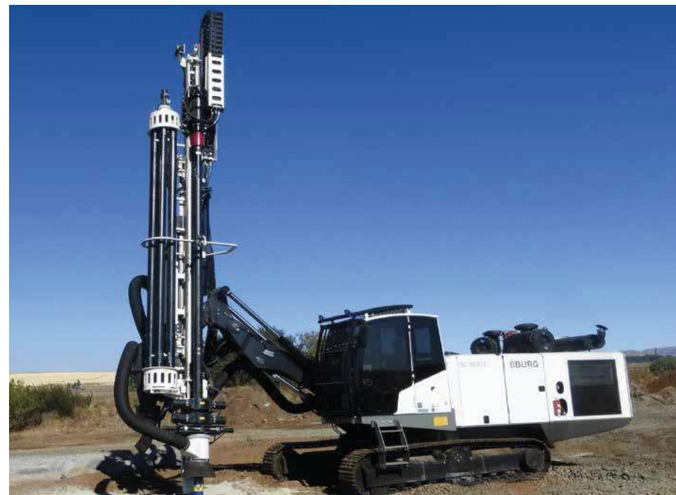
igus® E4.1 in an earth drilling machine. This vertically standing installation works even under strong vibration and harsh environments due to its plastic construction and having no loose parts such as rivets or screws
