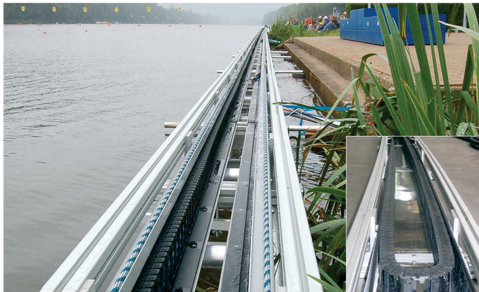
Long travel length with side-mounted orientation using the low noise and vibration series E6 for a camera application
