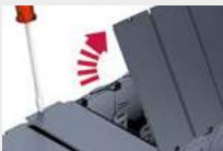
Simply unlock cover with a screwdriver
