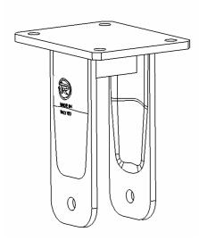
The bracket is made of a steel forged fixing top plate with 4 holes, of two steel drawn sides and of a central steel stiffener. These elements are secured by welding and properly protected against oxydation.
