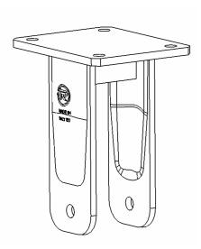
The bracket is made by a steel forged fixing plate with 4 holes, by two steel drawn sides and by a steel central stiffening. These elements are bounded by welding and properly protected against oxydation.
